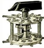
These switches can be made with any number of contact points up to fifteen, shorting or non-shorting, can be furnished with suitable insulation for metal panels, ganged in two or more decks, ¼" shaft, single hole mounting. Ideally suited for band switching, high resistance volt-meters, multi-range instruments, etc.
